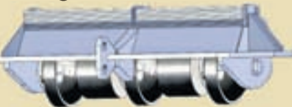
The new-type multi-rig clump for Morgère reduces seabed contact.
