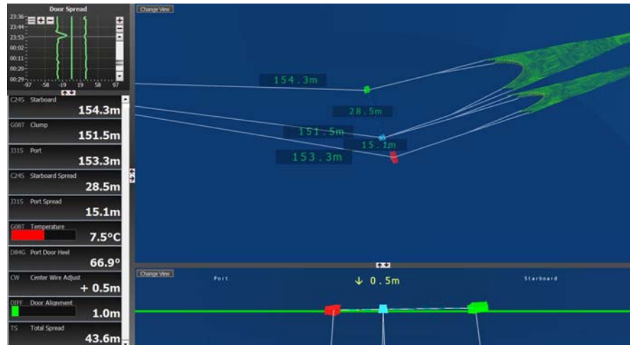
The above graphic indicates that the port door as fallen over (72.1°) and the port net has closed with only 14.2 m of spread.
